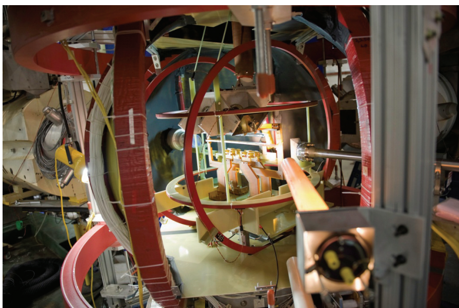
FIGURE 2.5.1: Photograph of Jefferson Laboratory's polarized helium-3 target, used to make precision electron scattering measurements of the charge, magnetism and spin distributions of the neutron. SOURCE: Courtesy of Thomas Jefferson National Laboratory.
